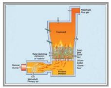
As the sludge enters the incinerator the heated fluidized sand hits the sludge both breaking it apart like a sand blaster and
